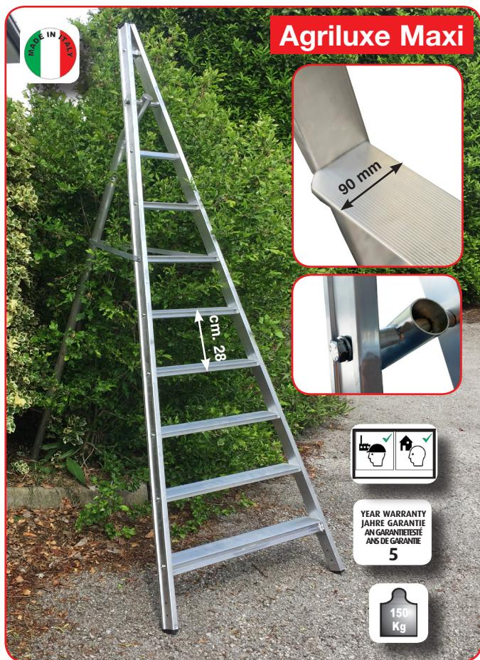
**EN** In ribbed extruded aluminum with converging uprights and pole which also allows for self-supporting position. The ladder can also be leaned against the tree. The non-slip knurled steps are fixed to the uprights with screws. The converging shape allows it to fit easily between the branches of the tree.
