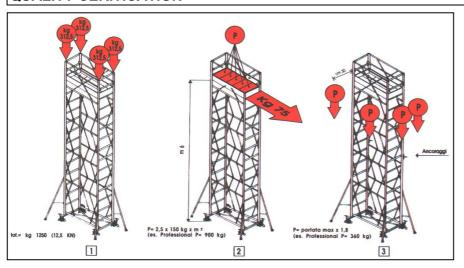
This Svelt scaffolding has been tested by engineers of the Politecnico di Milano according to the EN 1004 standards.
