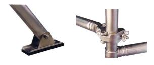
Locking of the braces by means of quick-connect hooks: all the crosspieces and parapets are equipped with quick-coupling hands that automatically lock onto the tubular structure. The design allows a contact surface of over 225 ° for a perfectly rigid scaffolding. The head of the "rhino horn" coupling makes the aluminum casting impact resistant in the event of a fall.
